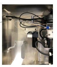
2. Disconnect the ribbon cable from the optical board.
