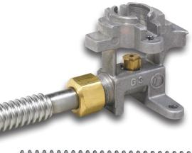
To enhance speed and ease of assembly, the nut and ferrule compression fitting is attached to the compression tube before shipment. The NF series of compression FlexTube arrives at the assembly line with the tubing ready to be attached to the valve or fitting. No fumbling with small ferrules, just hand thread the nut and tighten.
